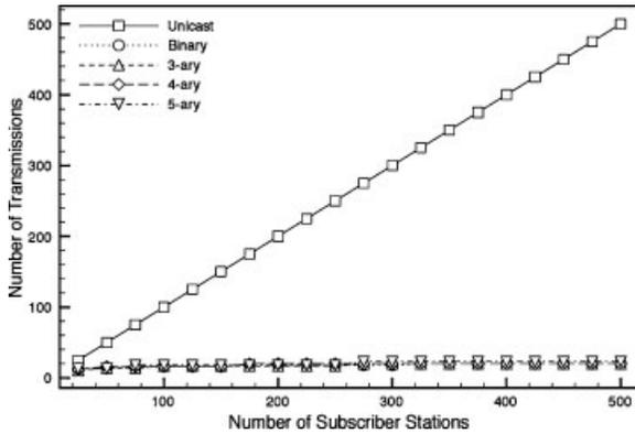
Fig. 6. Comparison of the total number of transmissions.
