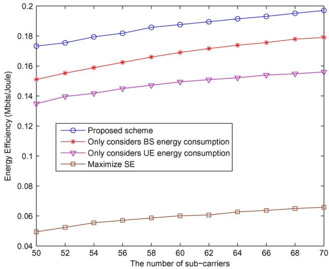
Fig. 7. EE of different resource-allocation schemes versus the number of subcarriers ( $\bar{\gamma}_2 = 15$  dB).
