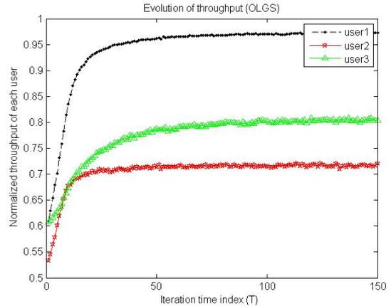
Fig. 4. Evolution of the throughput of each secondary user
