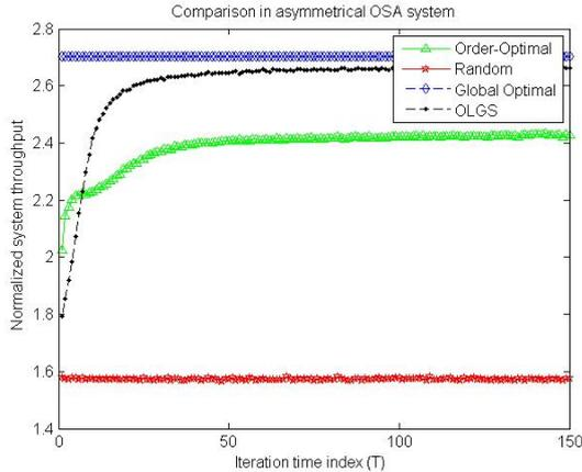
Fig. 3. Comparison of normalized system throughput of various schemes in an asymmetrical OSA system
