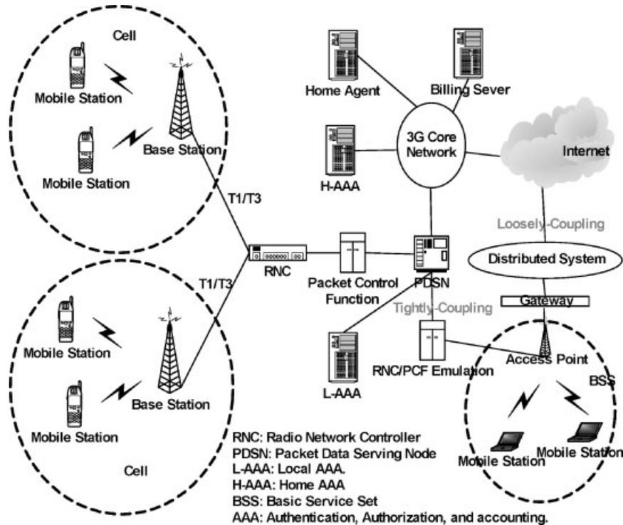
Fig. 2. Tightly-coupled and loosely-coupled in CDMA2000.
