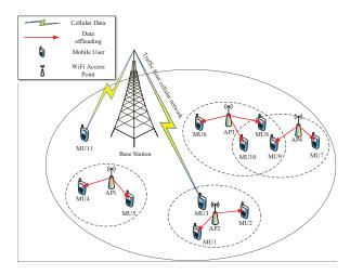
Fig. 1. Network scenario of WiFi offloading.
