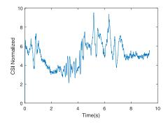
Fig. 12. CSI data processed with Butterworth filter.
