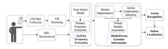
Fig. 14. Procedure of multiperson indoor localization.
