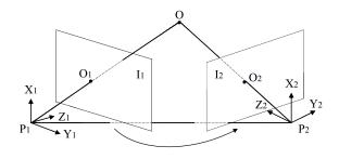
Fig. 1. Target localization model based on two images.
