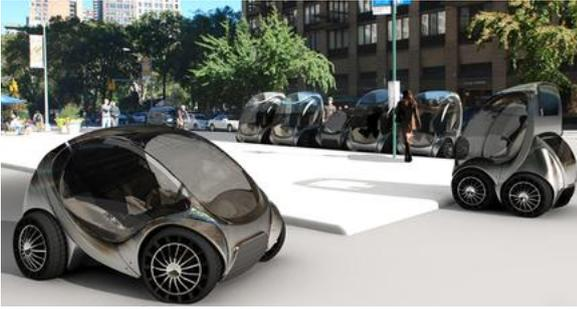
**Fig. 13** The vision of folded cars in the MIT’s CityCar project [40].
