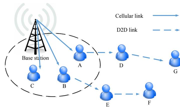
Offloading with mobile nodes
