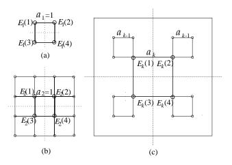
Figure 3. The recursive definition of eyes of (a) a  $2 \times 2$  mesh, (b) a  $4 \times 4$  mesh, and (c) a  $2^k \times 2^k$  mesh.
