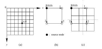
Figure 1. (a) A mesh with its coordinate system. (b) Broadcast in a  $2 \times 2$  mesh. (c) Broadcast in a  $4 \times 4$  mesh.
