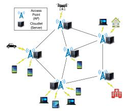
Fig. 1. An illustrative example of an MEC network consisting of 6 APs with each co-located with a cloudlet.
