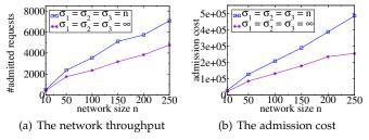
Fig. 8. Impact of the admission control policy on the performance of  ${\tt Algorithm}\ 3.$
