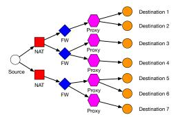
Fig. 2. An example of an NFV-enabled multicast request with a service function chain that consists of three network functions: Network Address Translation (NAT), Firewall (FW), and Proxy. Its data packet traffic flows from the source node *Source* to a set of seven destination nodes. Each packet must pass through one VNF instance of each of the three network functions in the service function chain.
