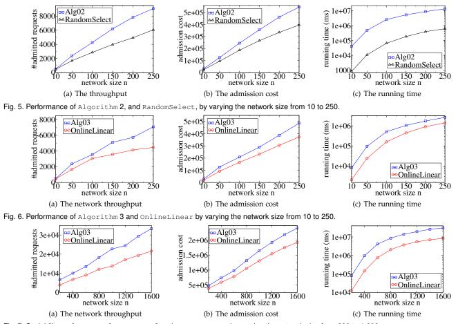
Fig. 7. Scalability performance of Algorithm 3 and OnlineLinear by varying the network size from 200 to 1,600.
