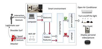
Fig. 1. Scenario of Secure Interaction with WiFi-enabled IoT environment
