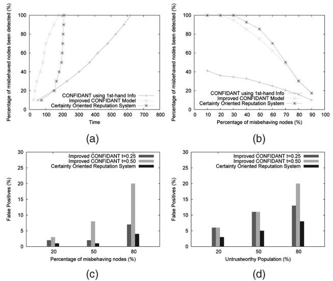
Fig. 6. Detection efficiency (a) over time, (b) with increasing percentage of misbehaving nodes; false positives when misbehaving nodes adopt (c) honest recommendation, and (d) bad mouthing and false praise.
