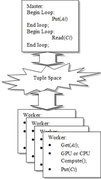
Figure 4. Logical View of SPP Programming.
