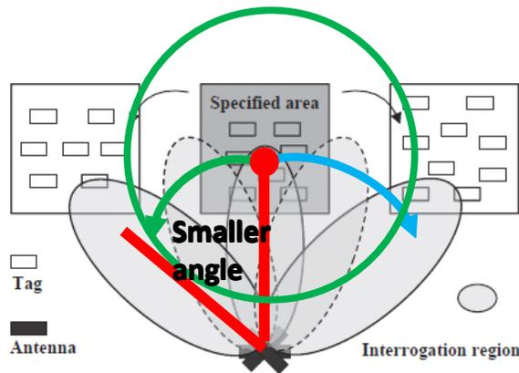
Fig. 5. Identify the tags in the specified area without any auxiliary equipment
