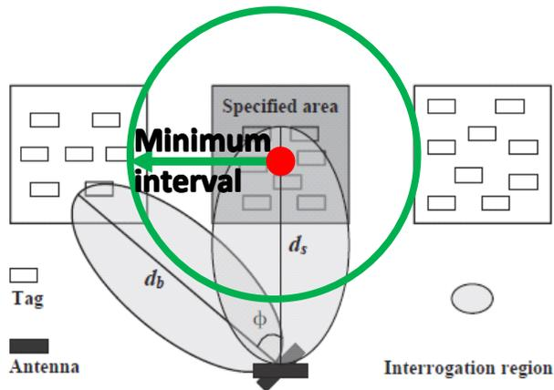
Fig. 4. Identify the tags in the specified area with a 3D camera
