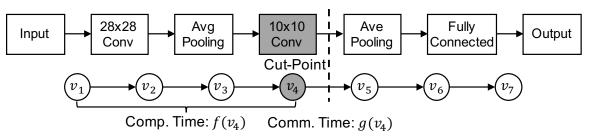
Comp.: forward propagation before cut-point layers Comm.: send outputs of cut-point layers
