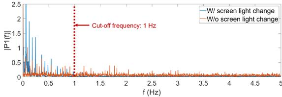
Fig. 6. The spectrum of luminance signals w/ and w/o screen light change.
