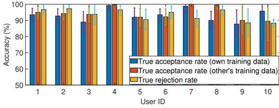
Fig. 11. Overall performance for a single detection.
