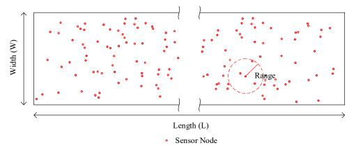
**Figure 1.** Illustration of a thick linear sensor network. Sample parameter values: L = 10,000 m, W = 500 m, and range = 100 m.
