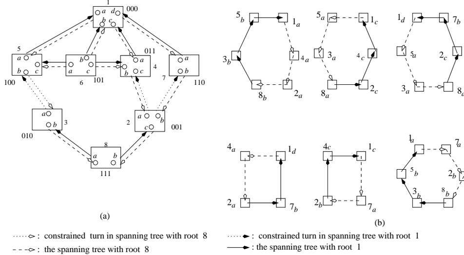
Fig. 2. Cyclic channel dependencies in an irregular network with STs: (a) the irregular network with input ports, and (b) the cyclic dependencies.
