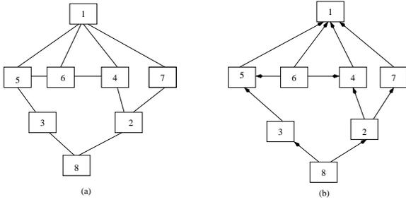
Fig. 1. An irregular network with a single ST: (a) the irregular network with eight nodes, and (b) the ST for up\*/down\* routing.
