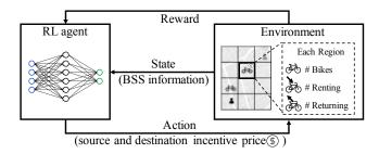
Fig. 3 An overview of the reinforcement learning framework.
