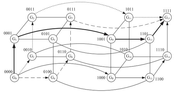
Fig. 4. An example of hypercube-based routing from  $G_0$  to  $G_{15}$ , where the directed lines are the multiple node-disjoint paths.
