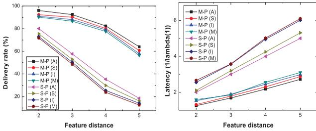
Fig. 10. Comparison of the performance between *multipath* and *single path*: (L): delivery rate and (R): latency. (M-P: multipath, S-P: single-path; A: analysis, S: synthetic, I: Infocom, and M: MIT.)
