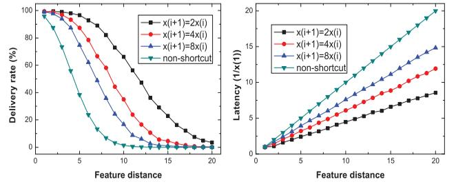
Fig. 6. Comparison between nonshortcut and two-hop shortcuts including in the single-path case. ( $x(i)$  is  $x_j^i$  for  $\forall j$ .)
