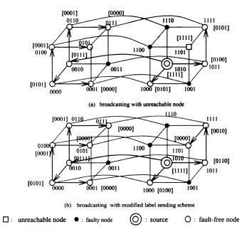
Fig. 2. Avoid forwarding message and label to nodes with at least 2 faulty neighbors in the BSC.
