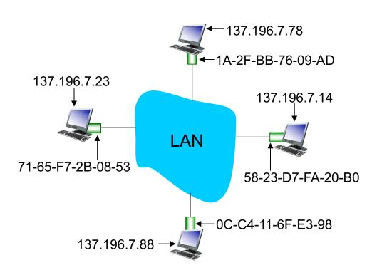
ARP table: each IP node (host, router) on LAN has table
