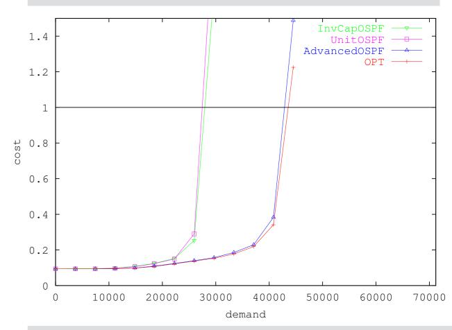
results on an AT&T backbone with a projected traffic matrix
