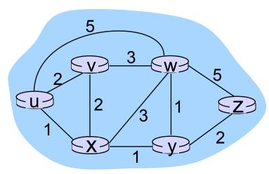
clearly,  $d_v(z) = 5$ ,  $d_x(z) = 3$ ,  $d_w(z) = 3$ B-F equation says:  $d_{u}(z) = \min \{ c(u,v) + d_{v}(z),$  $c(u,x) + d_{x}(z),$  $c(u,w) + d_w(z)$  $= \min \{2 + 5,$ 1 + 3, 5 + 3 = 4 node achieving minimum is next
