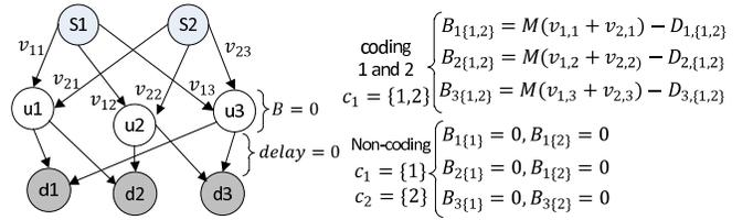
Fig. 8. A reduction from an instance of a vector packing problem to an energy-efficient broadcast with deadline constraints. ( $B_{j,c}$  represents the decoding delay for the packets of the set  $c$  at node  $d_j$ .)
