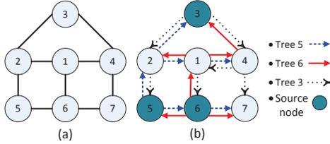
Fig. 2. (a): A given topology. (b): Two broadcasting trees
