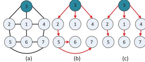
Fig. 3. (a): A given topology. (b): Broadcasting tree constructed using *Rule<sub>1</sub>* and *Rule<sub>2</sub>*. (c): Shortest path tree.
