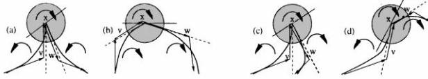
Fig. 16. A regular point (b) and three inflection points (a), (c), and (d).
