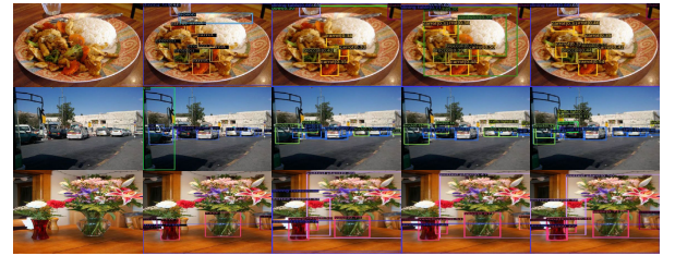
Fig. 7. Visual examples of qualitative detection results to evaluate the contribution of each component. From left to right are the input image, corresponding ground truth, predicted results from LRP, LRP + HRP, and full DPNet. For clarity, the estimated bounding boxes and associated labels are also superimposed on detected objects. (Best viewed in color.)
