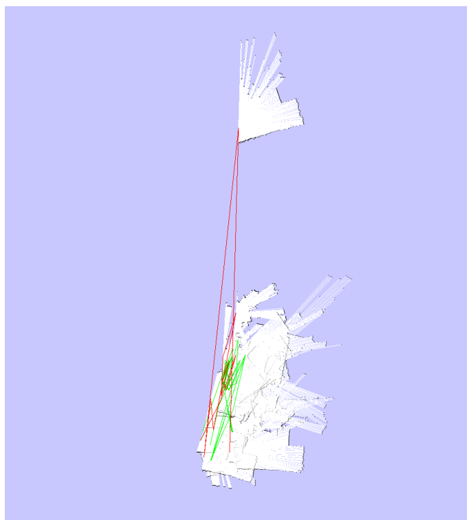
Figure 6.12: Map of the home environment computed by GMapping.
