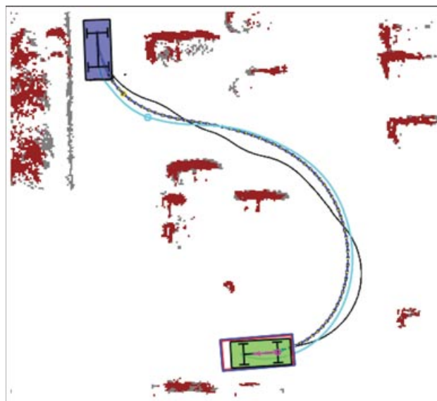
Figure 17. Path smoothing with conjugate gradient. This smoother uses a vehicle model to guarantee that the resulting paths are attainable. The hybrid A* path is shown in black. The smoothed path is shown in blue (front axle) and cyan (rear axle). The optimized path is much smoother than the hybrid A* path and can thus be driven faster.
