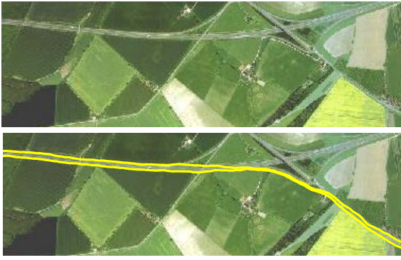
Figure 11. Tracking of road with width variations. Using simple first-order dynamics on the width, sampled simultaneously with the position dynamics, enables roads with varying width to be tracked.
