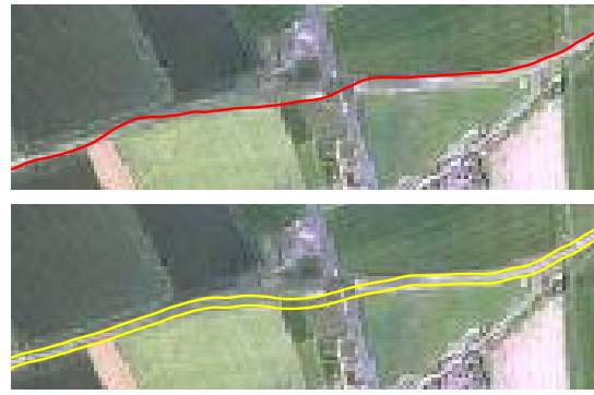
Figure 9. Extracting roads with ribbon model. Using a ribbon-like extension of contour model enables a stable extraction of roads, even with fixed width in this example.
