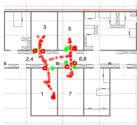
Fig. 10. Map displaying the robot path. The robot traverses four rooms crossing a corridor each time it moves from one room to another. Green (lighter)/red (darker) circles indicate the doors detected. The red (darker) circles also serve as the place references for the place explored on crossing the door. The numbers indicate the sequence in which the places were visited. The asterisks trace the actual path of the robot. (For interpretation of the references to colour in this figure legend, the reader is referred to the web version of this article.)
