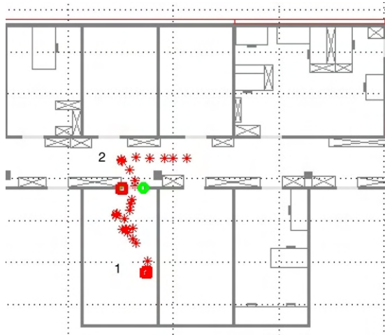
Fig. 13. The robot path for the experiment on reasoning about places. The robot traversed the path shown above. The configuration of the objects within the place was significantly changed from that in Fig. 11. The numbers indicate the sequence in which the places were visited. As before, a pair of circles represent a door detection. The red (darker) circles represent the reference for the place that is subsequently explored by the robot. (For interpretation of the references to colour in this figure legend, the reader is referred to the web version of this article.)
