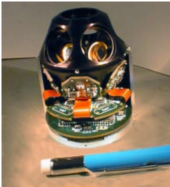
Figure 3: The HiBall is shown here with the internal circuitry exposed and the lenses removed. The sensors, which can be seen through the lens openings, are mounted on PC boards that fold-up into the HiBall upon assembly. The mechanical pencil at the bottom conveys an indication of the relative size of the unit.
