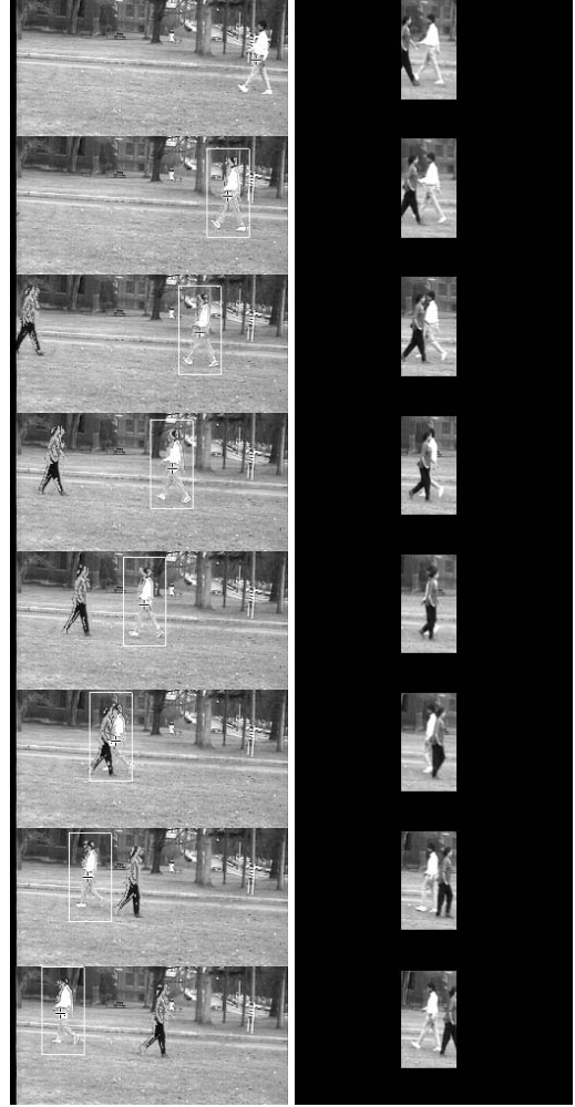
Figure 1: Left: Tracking applied to a walking person (every eighth frame shown); Right: image frames surrounding the interfering motion (consecutive frames)
