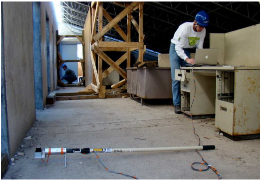
Fig. 7. Retrieving data in Disaster City. Photo of the scanned environment (the wall to the left appears at the top in Figure 8, the drawer (right) appears on the bottom of 8). The foreground shows the simple scan-tool, a stick-mounted laser.
