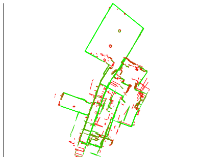
Fig. 12. A map of the same data set as Figure 11, created with deliberately mistuned parameters. Although, by visual inspection, it obviously models the reality worse than Figure 11(a), its evaluation value is higher due to its higher consistency. Please see text for explanations.
