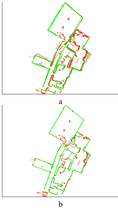
Fig. 11. Evaluation of two maps of the data set 'Freiburg082'. a) Quality of map \mathcal{M} = 0.2769 . b) \mathcal{M} = 0.4355 . Colors: level of green (vs red) shows confidence: The greener, the more confident, the more red, the worse. The higher regional confidence in (b) leads to the better total confidence value.
