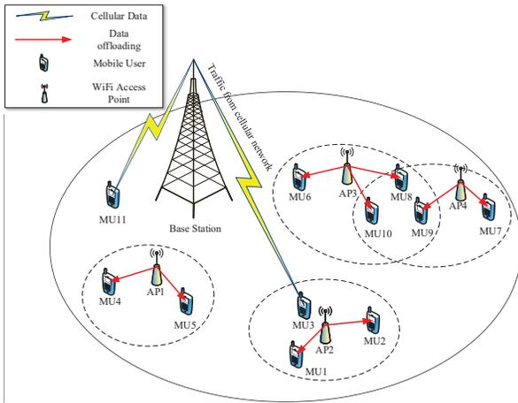
Fig. 1. Network scenario of WiFi offloading.
