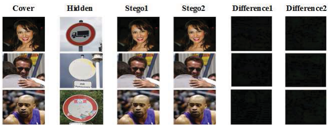
Fig. 2. Samples from the LSB substitution system. The 1 st column shows the cover images, the 2 nd column shows the hidden images, the 3 rd column shows the stego images with \zeta = 2 , the 4 th column shows the stego images with \zeta = 3 , the 5 th column shows the differences between cover images and stego images in the third column, and the 6 th column show the differences between cover images and stego images in the fourth column.
