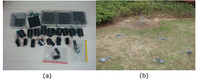
Fig. 2. (a) Solar motes used in our experiment; (b) The outdoor testbed.
