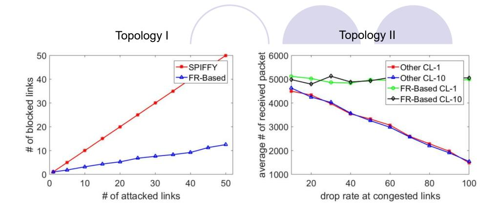
Number of blocked links are always less than SPIFFY The average number of receied packets is not affected by drop rate at links
