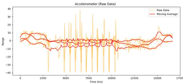
Figure 4. Accelerometer Graphed in Python (Moving Average Filter Applied)
