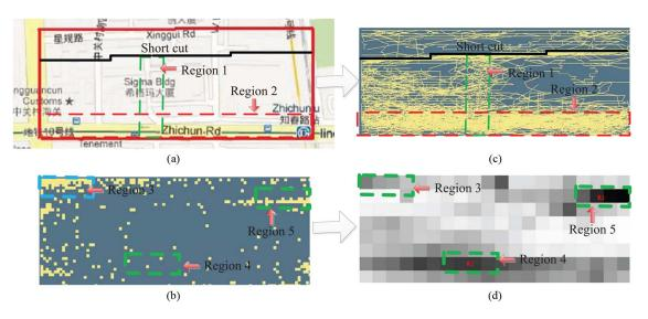
Fig. 3. Simulation setup and observations. (a) Simulation region (red rectangle). (b) Initial locations of mobile users. (c) User trajectories. (d) The possibility that a user stays in an area.
