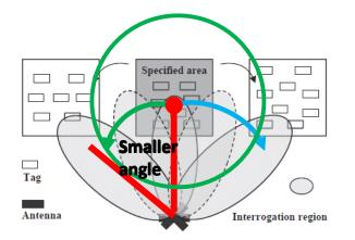
Fig. 5. Identify the tags in the specified area without any auxiliary equipment
