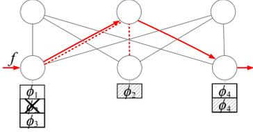
Fig. 4: Deployment of an SFC with backup instances.
