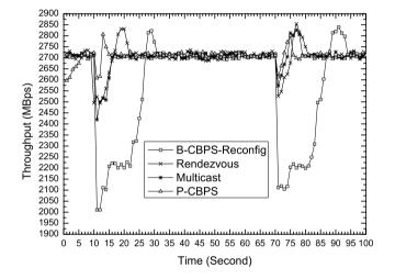
**Fig. 14.** The aggregate throughput of the system calculated in a 1 s time window a large network of 1000 brokers using different protocols.
