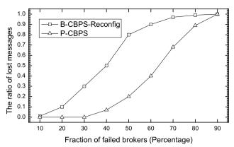
**Fig. 19.** The ratio of lost messages in a network of 100 brokers. The percentage of failed brokers varies from 10% to 90%.
