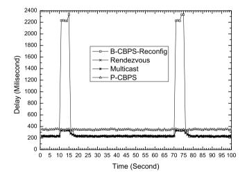
**Fig. 18.** The average delay of the delivered messages calculated in a 1 s time window in a network of 1000 brokers using different protocols.
