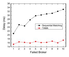
**Fig. 11.** The delay of delivered messages on the PlanetLab testbed with growing number of failed brokers.
