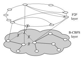
Fig. 2. High level illustration of the two-layer hybrid routing structure.
