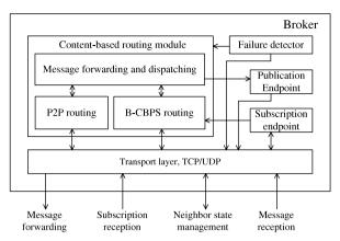
Fig. 8. High-level software architecture of a broker.
