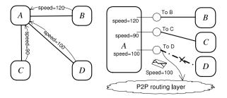
**Fig. 4.** The routing table of broker *A* is configured to forward the message to the matched brokers of each subscription. Traffic will be redirected to the P2P routing layer if failure occurs.
