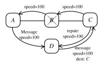
**Fig. 5.** Illustration of the rendezvous-based repair. Broker *B* failed. Broker *C* and *D* are the affected brokers. Broker *C* requests repair from the rendezvous broker *D*. *D* then forwards messages to *C* by using DHT routing. Arrows indicate the direction of message forwarding.
