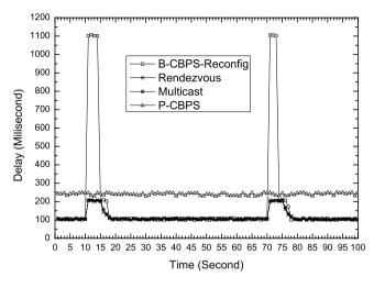
**Fig. 17.** The average delay of the delivered messages calculated in a 1 s time window in a network of 100 brokers using different protocols.
