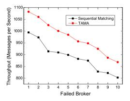
**Fig. 12.** The throughput on the PlanetLab testbed with growing number of failed brokers.
