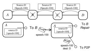
**Fig. 6.** Illustration of the multicast-based repair. Broker *A* knows the source of the subscription. When *A* detects that *B* failed, the interface to *B* is marked *repair*. Messages directed to the interface will be redirected to the P2P layer.
