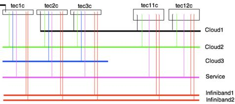
Cloud1 - GigE - All but tec1c connected - good for intra-VM communication Cloud2 - GigE - All nodes connected - good for NAT access and network file system access Cloud3 - GigE - All nodes 1U connected / No GPU systems connected unsure what we can utilize other than intra-VM's limited to these nodes Service - GigE on 1U systems/ 100Mb on GPU systems -
