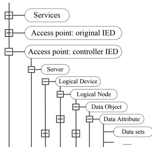
Figure 3. The architecture of the Data Model.
