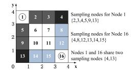
Fig. 1. An example of the partial sampling scheme.
