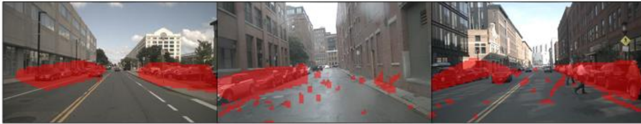
(a) Extracted foregrounds when vehicle is moving straight.
