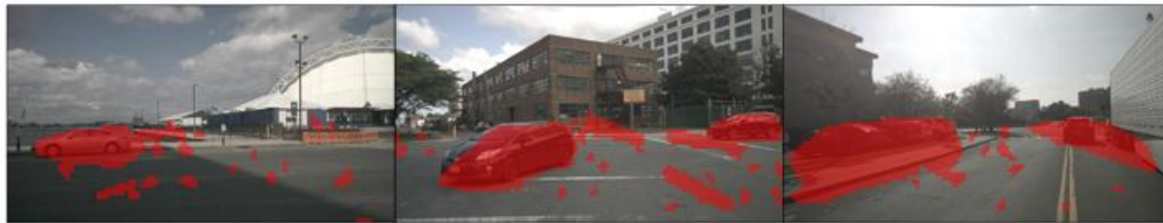
(b) Extracted foregrounds when vehicle is turning.
