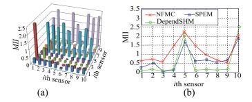
Fig. 11. (a) Distributed sensor fault detection (5th sensor and 10th sensor are faulty); (b) MII achieved by the two detection methods under the sensor faults.
