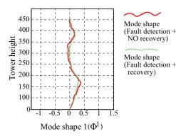
Fig. 8. Observation on the actual mode shape curvature vs. mode shape curvature in cases of faulty sensors and recovery (signal reconstruction).
