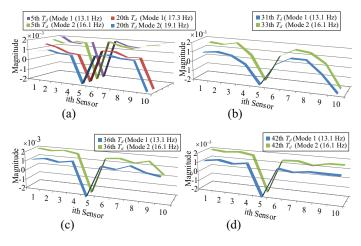
Fig. 12. The mode shape's curvature under sensor faults and recovery from the faults.
