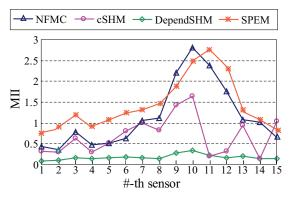
Fig. 6. Performance of different fault detection methods: achieved MII under sensor faults.
