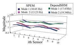
Fig. 10. Global mode shape  $(\Phi)$  curvatures based on each sensor individual frequencies in SPEM and DependSHM.
