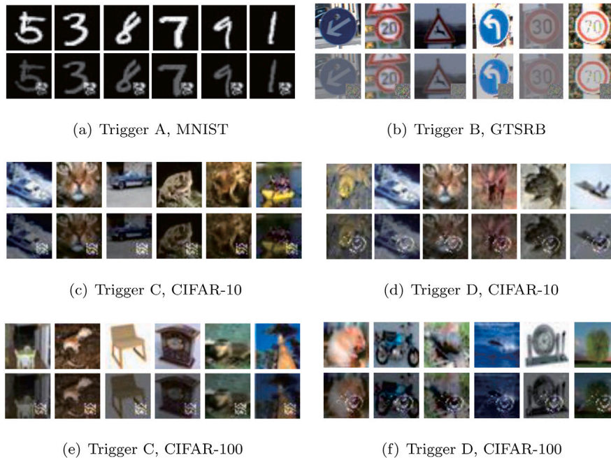
Fig. 7. Benign samples and their corresponding poisoned versions. Top row: Benign samples from different datasets. Bottom row: Poisoned samples transformed by CycleGAN.
